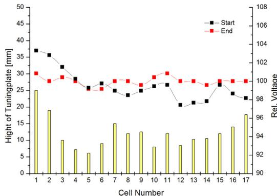
Figure 5: Relative longitudinal voltage distribution before (black) and after (red) the tuning. The bars show the positions of the tuning plates.
