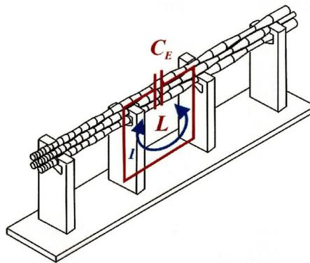
Figure 4: Basic cell of the 4-rod RFQ structure.
